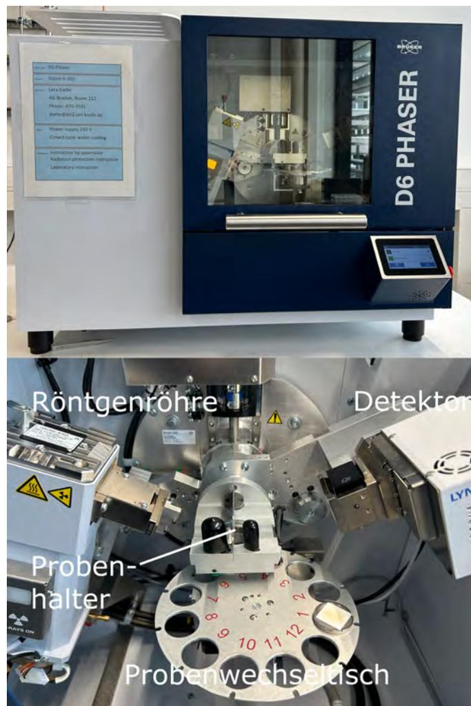
Figure 2.1: Röntgen-Diffraktometer Bruker D6 Phaser.
