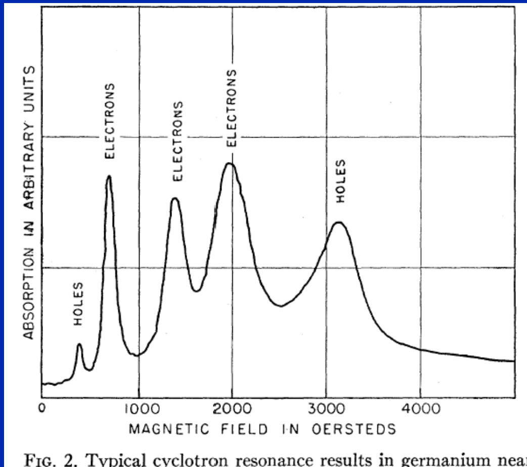
FIG. 2. Typical cyclotron resonance results in germanium near
