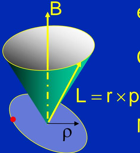
$e^-$  in  $B$ -field  $\Rightarrow$  Larmor precession with  $\omega_L = \frac{eB}{2mc}$
