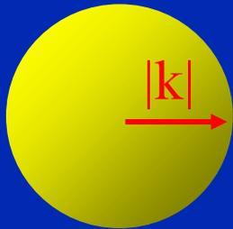
$$N(|\vec{k}|) = \frac{V_{\text{cell}}}{(2\pi)^3} \frac{4\pi}{3} |\vec{k}|^3$$
