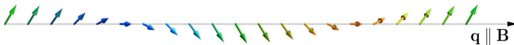
Figure 7: Alignment of the propagation vector \mathbf{q} along the direction of the applied magnetic field [37].
