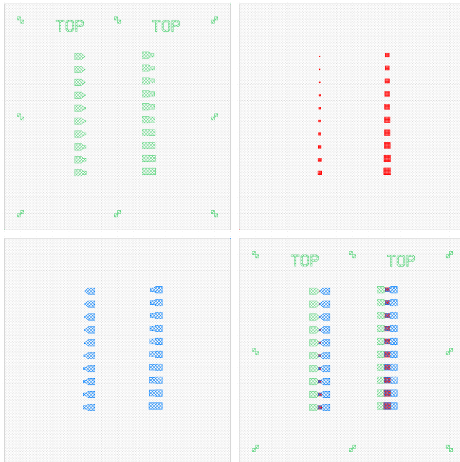
Fig. B.1: from top left to bottom right: gold bottom layer (green); HfO x intermediate layer (red); gold top layer (blue); whole chip design
