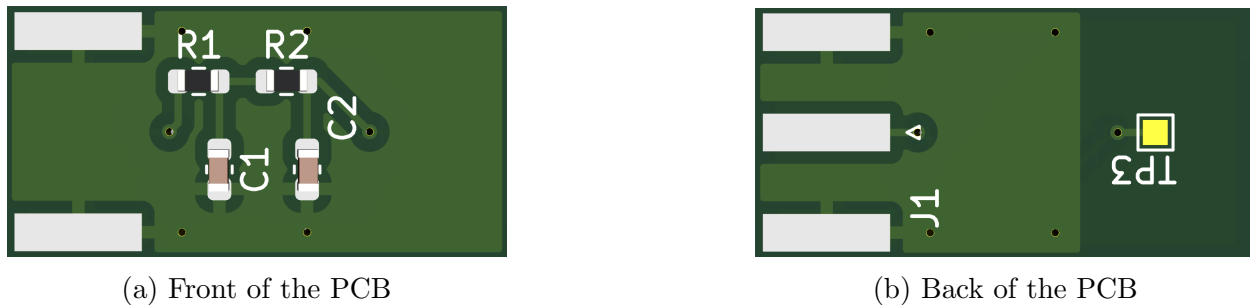
Figure 15: Final design of the PCB. The components are marked with the respective Symbol (see figure 14). The light green space is a conductive surface and sets the ground potential for most of the PCB. The front and back sides are connected via holes. The yellow surface is a soldering spot. The silver spots are soldering attachments to a female SMA connector. [18]
