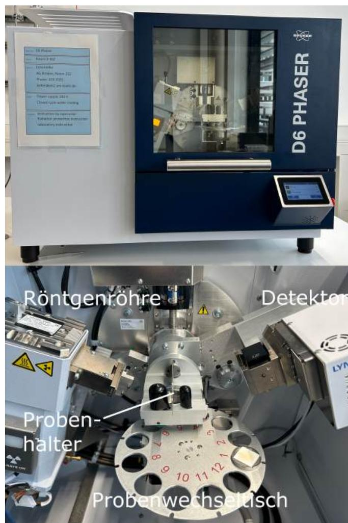
Figure 2.1: Röntgen-Diffraktometer Bruker D6 Phaser.
