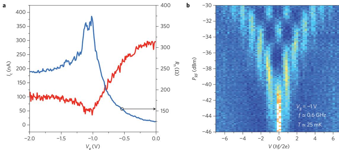
**Figure 4 | Shapiro response of a junction on a trivial quantum well.** **a**, Critical current  $I_c$  and normal state resistance  $R_n$  of a non-topological device as a function of gate voltage  $V_g$ . **b**, 2D map of the voltage distribution as a function of the d.c. voltage (in normalized units) and the RF excitation power  $P_{RF}$ , taken at  $V_g \approx -1$  V and frequency  $f = 0.6$  GHz. At this frequency, close to our resolution limit, all the steps are still visible.
